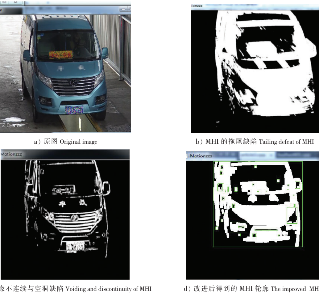
图 1 运动历史图性能对比 Fig.1 Comparison between improved MHI and original MHI
