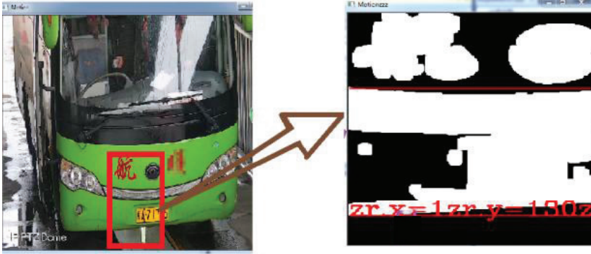
图 5 镜头抖动时目标区域内检测到的车体轮廓特征 (存在横跨区域水平线) Fig.5 The vehicle contour detected in the target area when lens jitter with vehicle (get crossing horizontal line)
