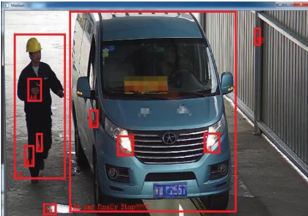
图 2 运动检测中行人及水坑的干扰 Fig.2 Disturbance from pedestrians and puddles in motion detection
