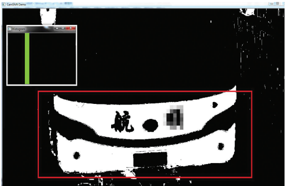
图 6 目标车体颜色直方图及当前帧车体轮廓 Fig.6 Target vehicle color histogram and the car contours of the current frame
