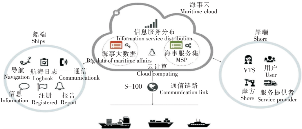
图 2 “海事云”网络架构 Fig.2 The network architecture of “maritime cloud”
