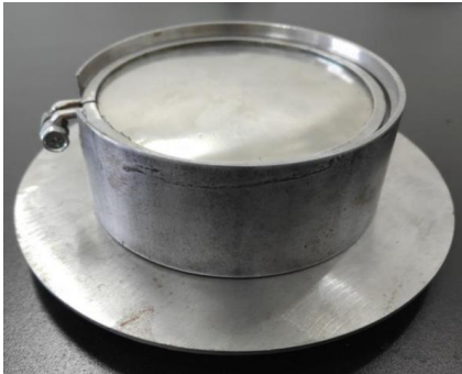
图2 屈曲板型高静低动隔振器实物样机 Fig.2 The prototype of buckling plate type high-static-low-dynamic stiffness vibration isolator
